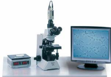
Fig 7a: A high powered microscope connected to a monitor screen so that semen samples can be analysed by a number of people at the same time.
