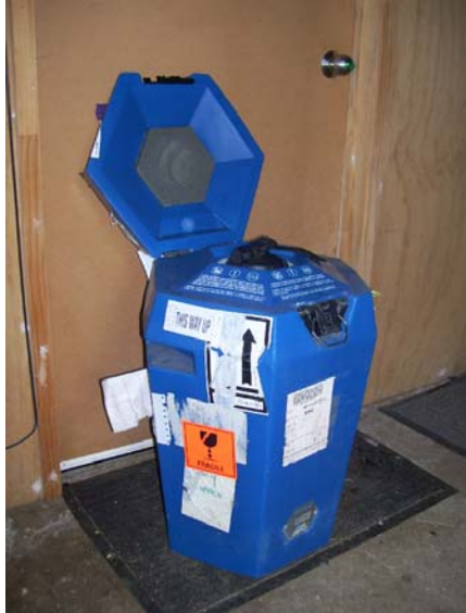
Fig 3: This is a picture of a “dry shipper” container used to transport frozen semen all over the world.
